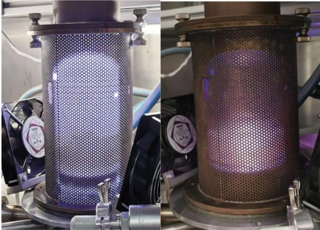
A reproducible etching rate of **80 nm/min** was found in O<sub>2</sub> plasma at 300 W power, 0.3 mbar pressure.
