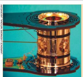
A hohlraum made from gold and 1 cm tall contains the fusion fuel capsule used in experiments at the National Ignition Facility. Light from the laser enters the ends of the cylinder and is converted to x rays, which implode the capsule.
