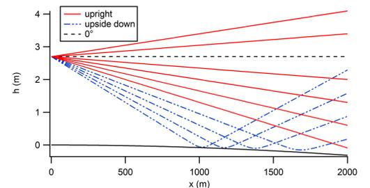
Bending of light rays in air over a water surface with ambient temperature 1°C and water temperature 5°C, on a distance of 2000m. Each ray starts from a height of 2.7m in different angles (-0.16-0.04°) from horizontal in 0.02° steps. The surface of Earth is indicated with a black curve.
