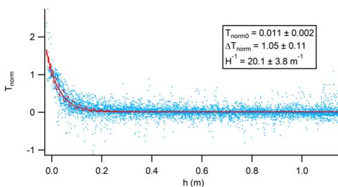
We **fitted** an **exponential** function on **normalized** measurement data (temperature as a function of height) of the form:
