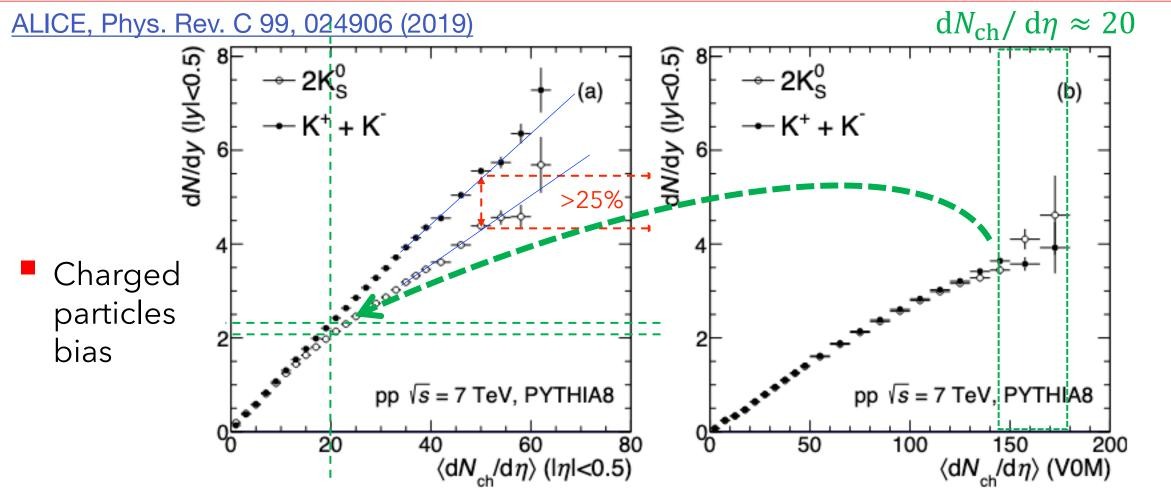
Better control of the biases when the multiplicity is measured in the V0 detector, but at the cost of a lower multiplicity reach ( $|\eta| < 0.5$ )
