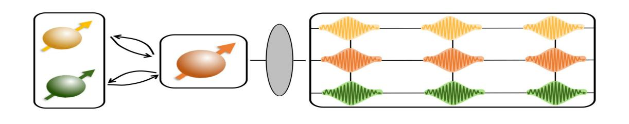
ST1 color center is a single photon emitter which was discovered in diamond nanowire. This center in diamond can be a long-living solid-state quantum memory. There was a hint from experiments to verify this oxygen-vacancy complexes with ab-initio calculations.
