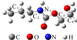
Figure 2. Optimized (B3LYP/6-311++G(d,p)) geometry of UDMA model (C 1 H 2 -C 2 H 2 and C 3 H 2 -C 4 H 2 groups are in anti and gauche conformational states, respectively).
