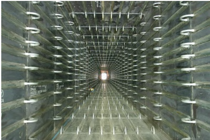
T2K decay volume (Helium filled, length: 110m)
