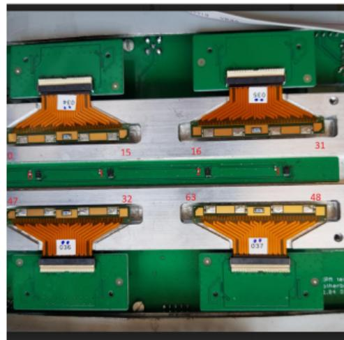
Place the arrays and start the test. IV low intensity light and dark, Single Photon Spectrum with pulses, plexi + optical cable under the SiPMs
