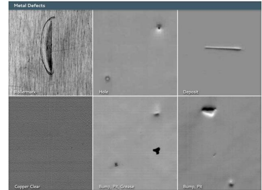
Fig. 1 Different types of surface the defects in metals
