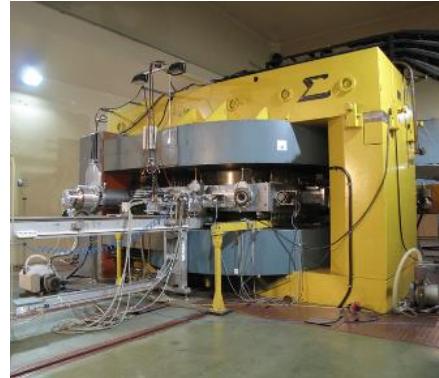
AIC-144 cyclotron protons 60 MeV
