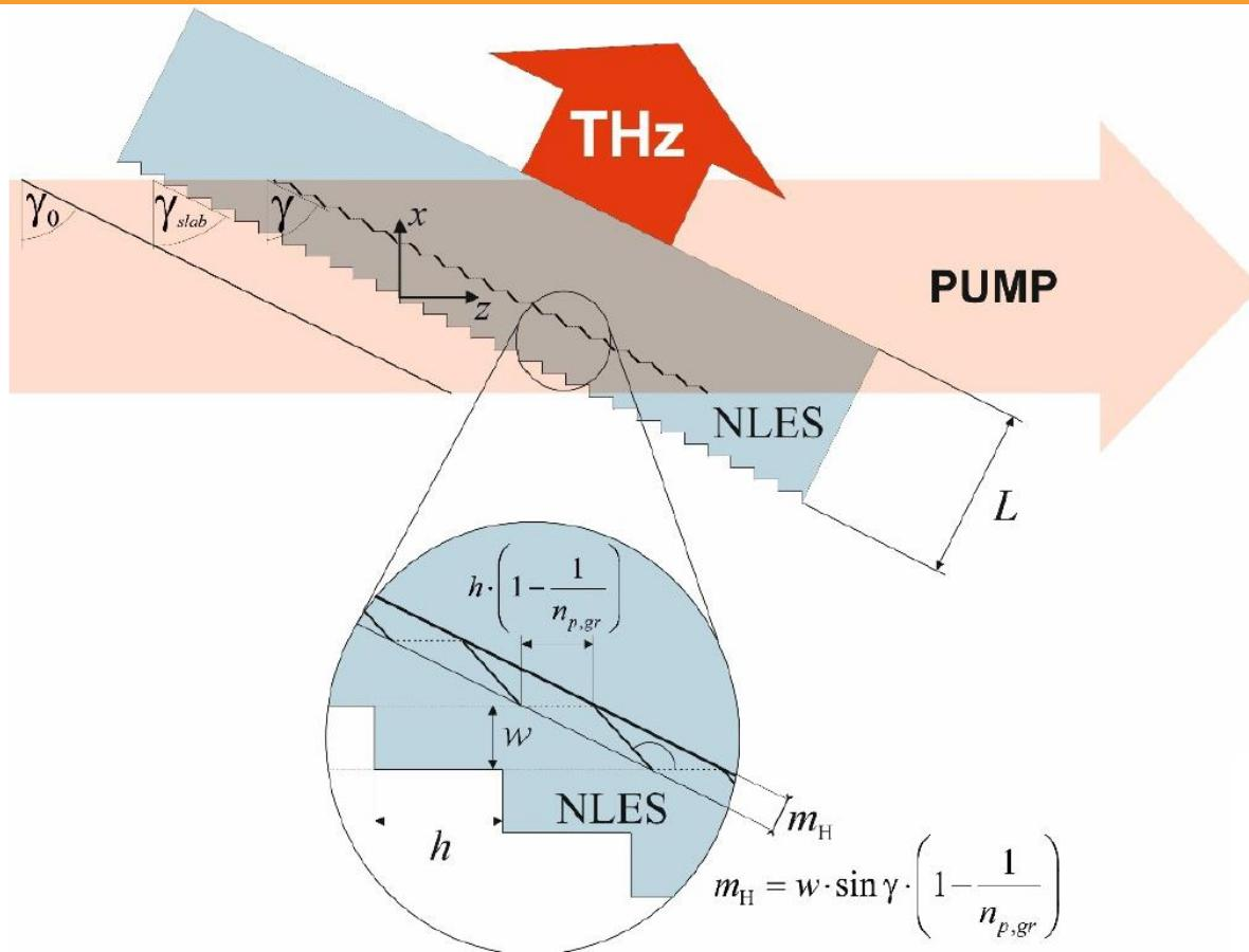
1 mJ THz predicted at  $T = 100$  K for 500 fs, 100 mJ pump from 1 inch diameter LN with  $\eta = 1$  %
