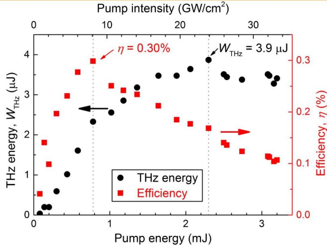
X100 efficiency compared to 800 nm pumped ZnTe
