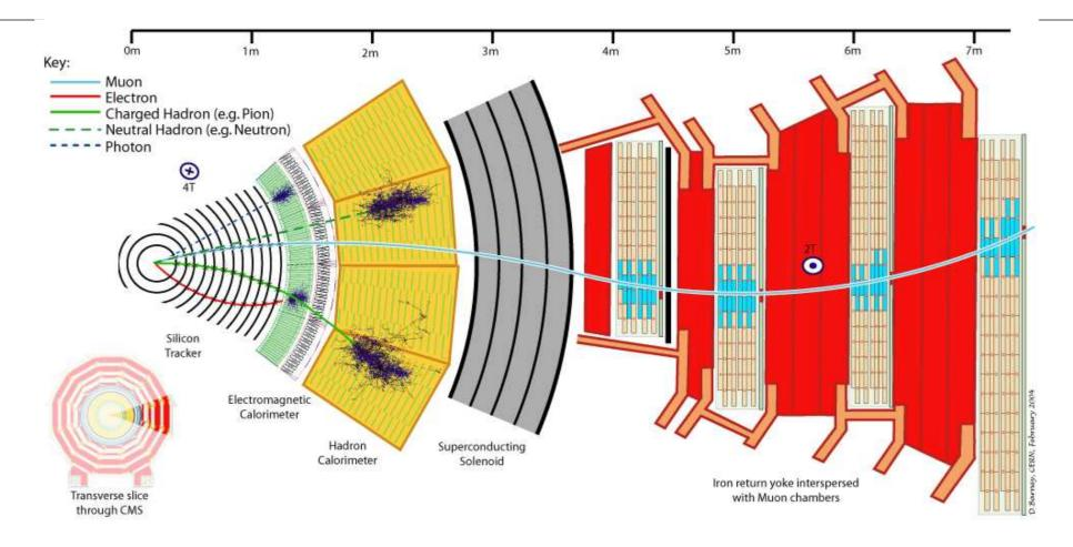
The fast muon flies through every part of the detector. The tracker follows its orbit in the 3.8 T magnetic field. The muons are selected by a muon trigger, but their transverse mmentum is measured by their orbit curvature using the silicon pixel and strips tracker.
