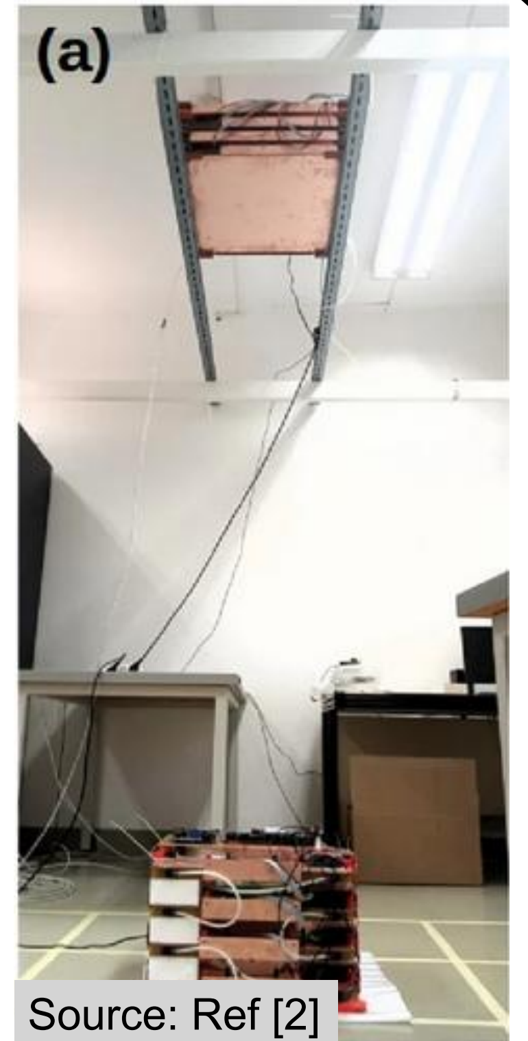
Reference (above) and Receiver (below) of the two-dimensional navigation system
