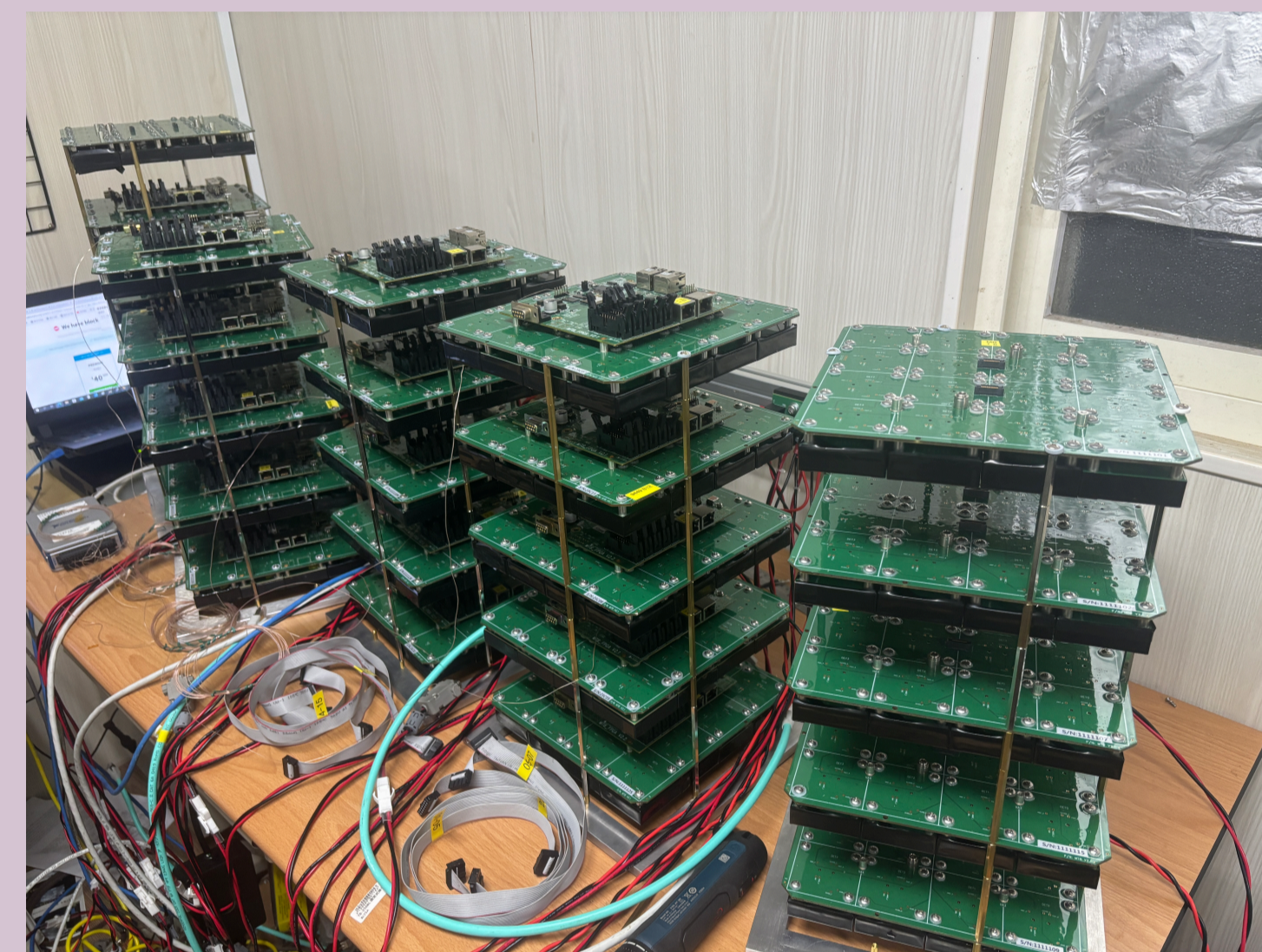
Fig.13 Setup of efficiency measurement
