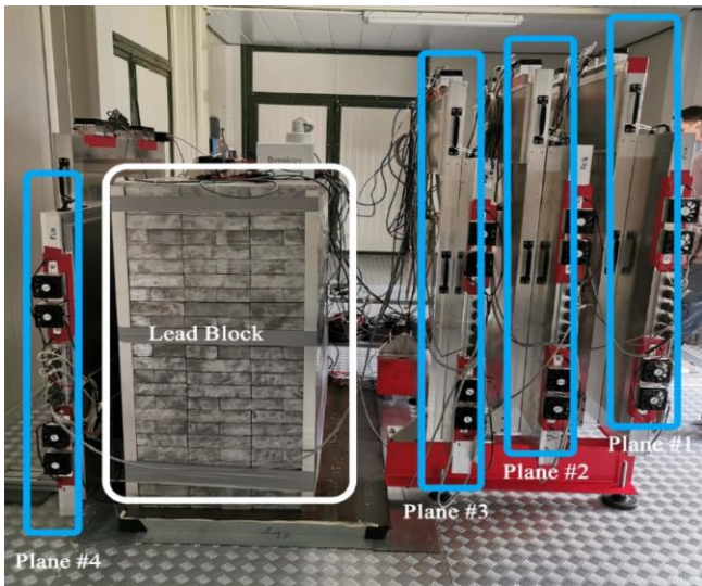
MURAVES hodoscope. Four scintillator station and the lead wall between 4 th and 3 rd plane is marked.
