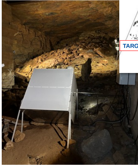
Rear view - D2 - Scintillator - "SC"
