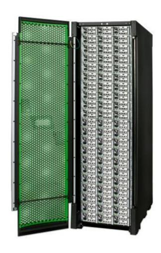
126x ATI Radeon HD5970 = 584 TFLOP SP
