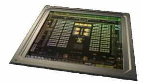
256 cores 1000 MHz base clock Maxwell-architecture
