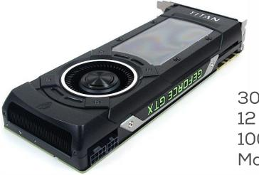
3072 cores 12 GB memory 1000 MHz base clock Maxwell-architecture
