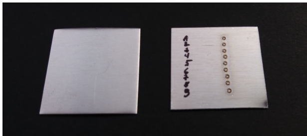
25 mm \times 25 mm Al-foils (200 \mu\text{m} thickness) before and after laser ablation
