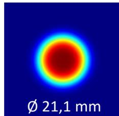
Propagated beam profile on the folding mirror
