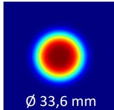
4th order supergaussian beam profile on lens 3
