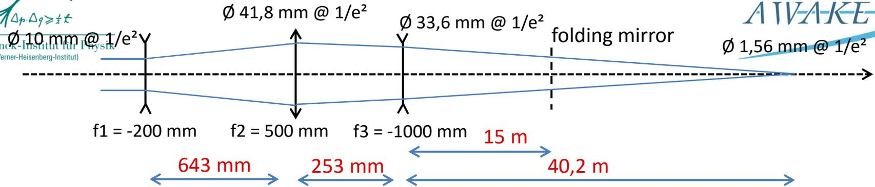
Effective propagation of the 10 mm beam to the folding mirror : 2,3 m
