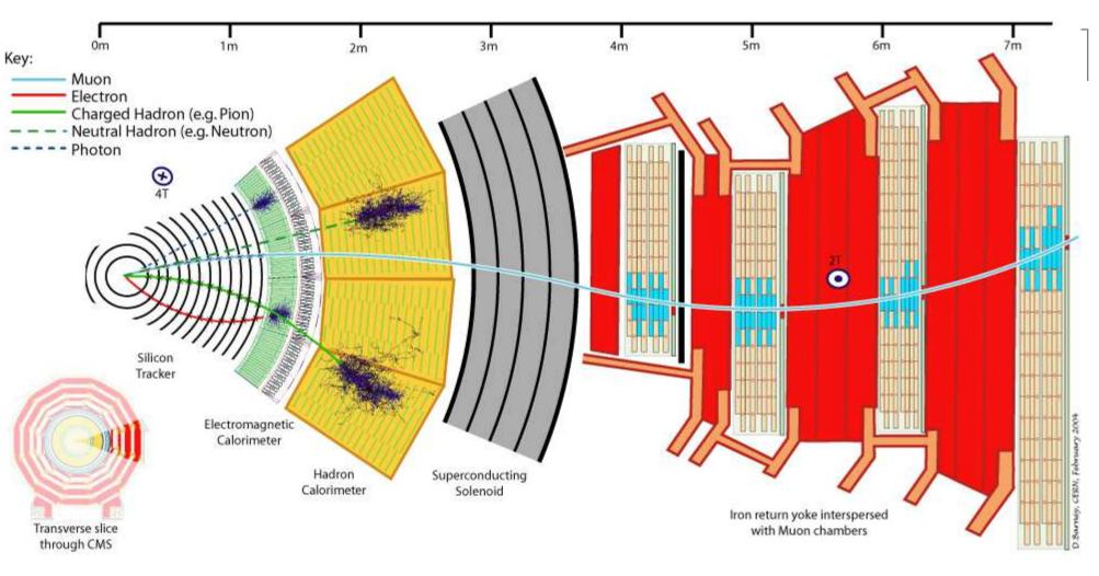
14000 ton digital camera: 100 M pixel, 20 M pictures/sec, 1000 GB/sec data Processes cc. 400 pictures/sec  $\Rightarrow$  intelligent filter!!
