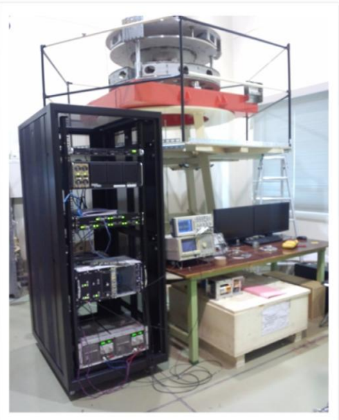
Prototype pre-isolator with the digital control system at ICRR
