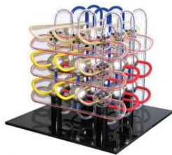
"6-dimensional mesh/torus" topology (model)
