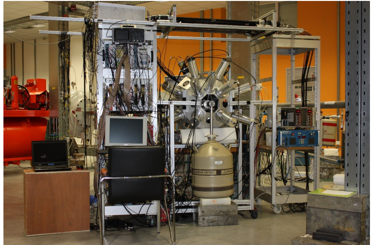
\gamma -spectrometer with twelve, 3"x3" and two 3.5"x6" LaBr 3 detectors
