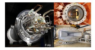
Fast cycling (4 Tesla /s) super conducting (s.c.) magnets incl. cryo-technology
