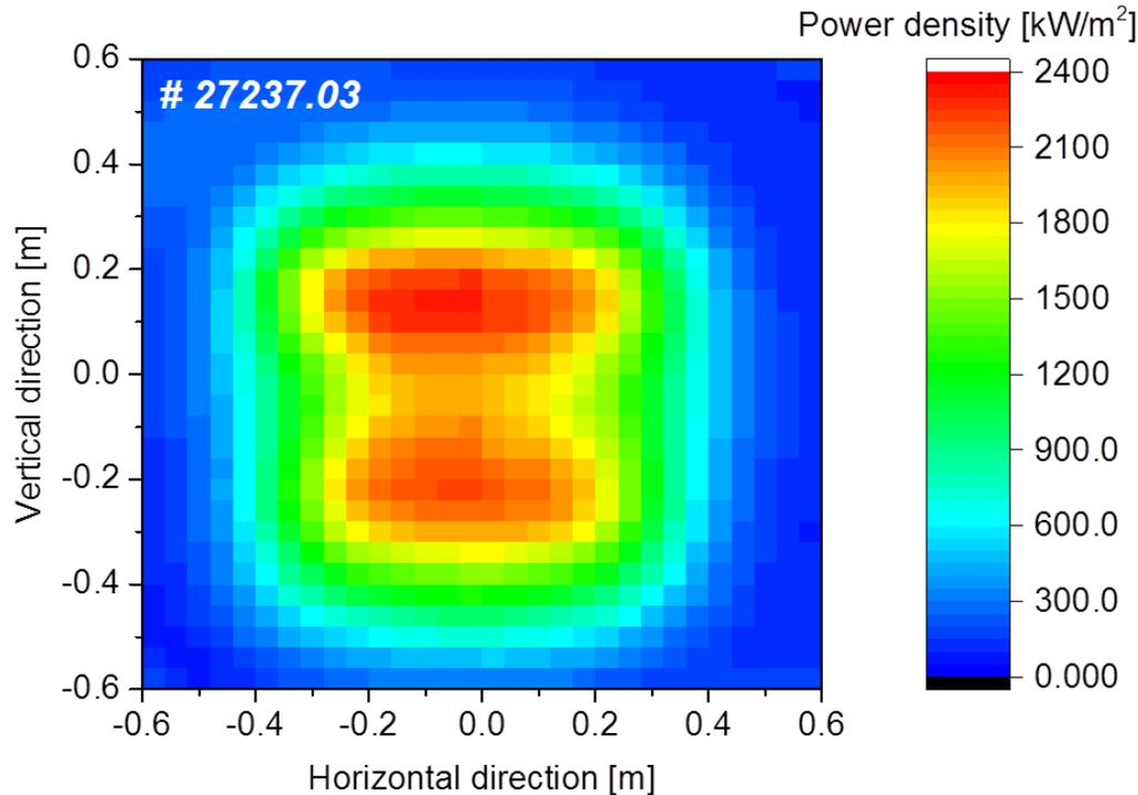
**23.8 A at the calorimeter (ITER value: 23 A)**
