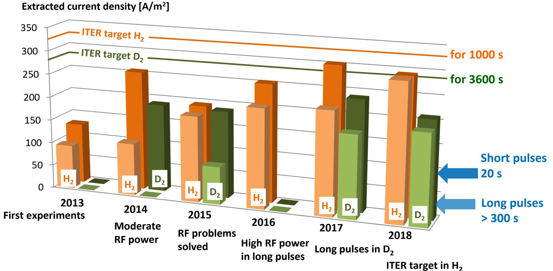
The source performance is limited by the amount of co-extracted electrons!
